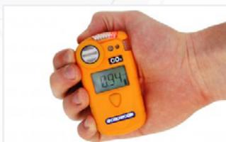
It stands out because of its infrared sensor technology, which ensures excellent stability, less interference and a very long service lifetime (>60 months).
