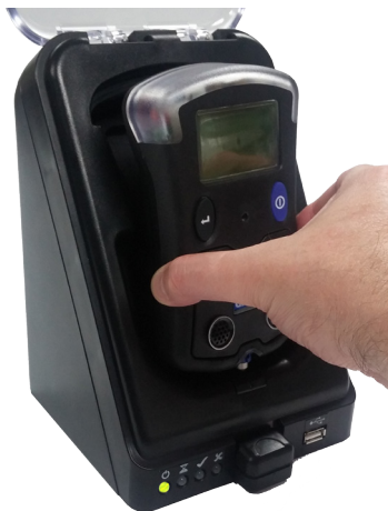
Fig. 4-11 Lift Instrument Clear of Gas Nozzle
