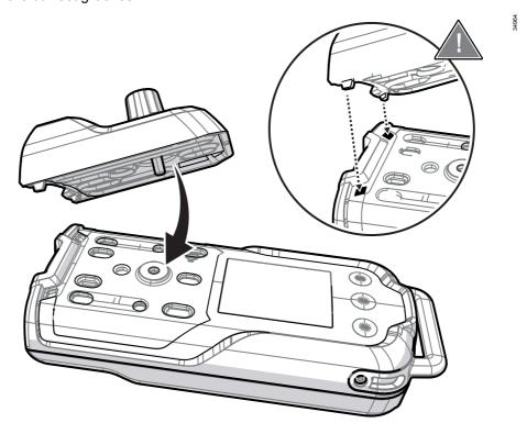
i Check that the pump adapter is mounted correctly. If the pump adapter is mounted correctly, the leak test starts automatically. If the leak test does not start, the gas detector is not ready for use. Avoid bending the pump adapter.
