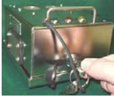
1. Activate the DS4 alarm by inserting the key into the switch and turning the key in a clockwise direction.
