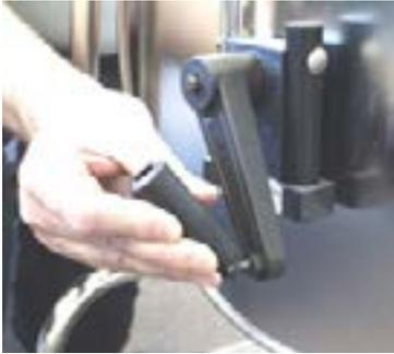
11. Firmly grasp and pull the winding handle knob away from the hose reel. Fold the knob against the handle.
