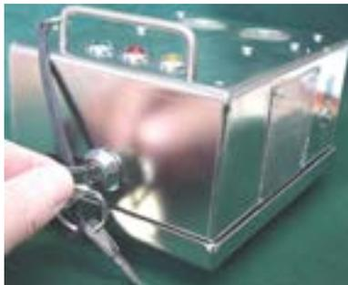
2. Switch off the DS4 unit by turning the key in a counter-clockwise direction.
