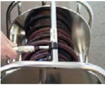
10. Connect the hose CEJN outlet to the parking connector on the hose reel. This prevents the hose unwinding and vents any pressure left in the medium-pressure circuit.
