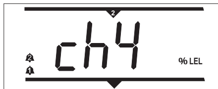
Figure 3.3 Example system in alarm
